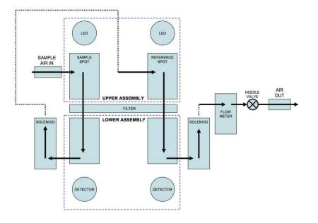
Figure 2: Schematic of the sample air flow within the TAP.
