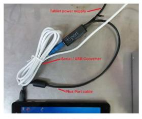
Figure 23: BMI Tablet/Plus Port Connection
